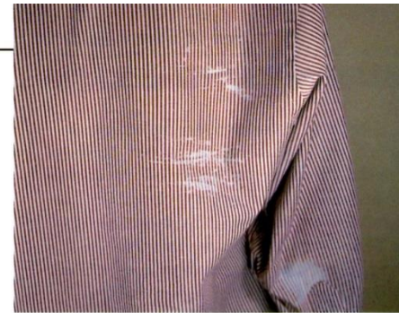
Some colored yarns in this shirt have been lost, causing the white area as shown.
